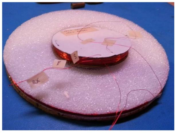
The above picture show the coil windings just before gluing the Rx coil spool in place. The coil windings must be secured so that no wires can move against one another. This can be accomplished by covering the windings with Cyan glue.. BUT, be very careful as too much Cyan glue can dissolve foam! A better solution is to fill the void around the Rx/Bx coil with epoxy. The same applies to the Tx windings. They must be secured with glue.
