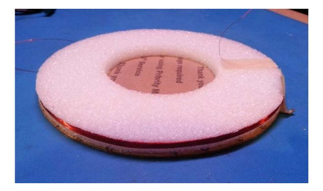
We will then wind 195 turns counter clockwise on the 43mm spool to create our Rx winding. Be sure to mark the beginning and end of the Rx windings.
