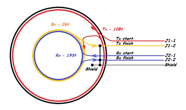
The important thing to note is winding direction and what end of the Tx coil is "hot" as this will affect coil nulling. The grounded end of our Tx coil must be closest to the Rx coil. Also note that the Tx and Rx coils are wound in the same direction, but the bucking coil (Bx) is wound opposite of the other coils. The Bx coil will be used to cancel the primary transmit field closest to the Rx coil. This is the way that we achieve "induction balance".
