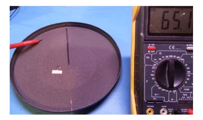
The top shell is shielded in the same manner with a drain wire of its own. The picture below shows the top shell before being sprayed. I will use an industrial strength double stick tape to secure my coil "sandwich" to the top of the shell . I just peel off the top layer of paper after graphite is applied to expose the sticky surface.
