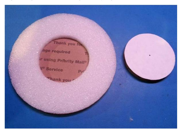
We will want to cut a small groove to accept our Tx winding on the 100mm form. To do this, you can use a hot soldering iron. You can cut the groove about 2.5 mm deep so that the final diameter of the Tx coil is about 95mm. Then, wind 105 turns of wire on the form counter clockwise. We can then test the running frequency by connecting it to the Tx circuit of the TGSL. It should run at 14.5kHz or just a bit lower. Later on when we add the bucking coil, the frequency will increase slightly.
