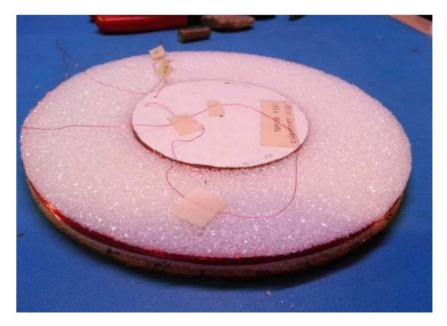
The USB-2 cable is fed through the BOTTOM of our coil arrangement and the leads are soldered. Then it will be time to do our final nulling adjustments. Quite simply, to null the coil, connect the Tx circuit to the TGSL. Connect a DVM (on the lowest A.C. setting) to the bare leads of the USB-2 cable going to the Rx coil. Turn the TGSL on and adjust the small wire loop to find the deepest null possible. Something less than 4mV should be achieved.
